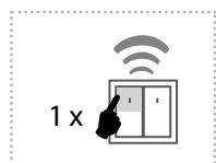
The output contact will be closed by pressing the button and opened after the set time interval has elapsed.
