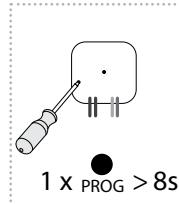
Bypressing the programming button on the actuator for 8 seconds, deletion occurs of the actuator's entire memory. LED flashes 4x in each 0.5s interval (max. 4 min.). The actuator goes into the programming mode, the LED flashes in 0.5s intervals (max. 4 min.). You can return to the operating mode by pressing the Prog button for less than 1s. The LED lights up according to the pre-set memory function and the component returns to the operating mode.
