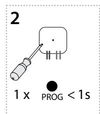
Pressing the programming button on the RFSA-x1B receiver for less than 1 second will finish the programming mode, this will reverse the memory function. The LED lights up according to the current pre-set memory function. The set memory function is saved.
