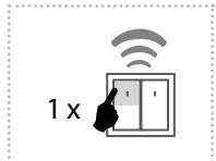
The output contact will be switched to the opposite position by each press of the button. If the contact was closed, it will be opened and vice versa.
