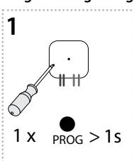
Press of programming button on actuator RFSA-11B for 1 second will activate actuator RFSA-11B into programming mode. LED is flashing in 1s interval.
