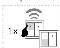
The output contact closes by pressing one button position, and opens by pressing the other button position.
