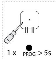
Bypressing the programming button on the actuator for 5 seconds, deletion of one transmitter activates. LED flashes 4x in each 1s interval. Pressing the required button on the transmitter deletes it from the actuator's memory. To confirm deletion, the LED will confirm with a flash long and the component returns to the operating mode. The memory status is not indicated. Deletion does not affect the pre-set memory function.
