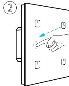
Pressing the programming button on the receiver for less than 1 second will finish the programming mode, this will reverse the memory function. The LED lights up according to the current pre-set memory function. The set memory function is saved. Every other change is made in the same way.
