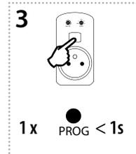
Press of programming button on actuator RFDSC-71 shorter than 1 second will finish programming mode. The LED lights up according to the pre-set memory function.
