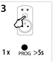
Press of programming button longer than 5 seconds, will activate socket into timing mode. LED flashes 2x in each 1s interval. After releasing the button, the time of the sunrise function begins to count down (period of complete illumination of the light).
