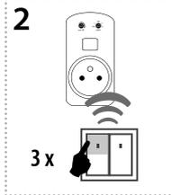
Three presses of your selected button on the RF transmitter assigns the function light scene 3 (must be a lapse of 1s between individual presses).
