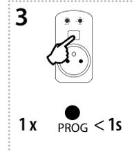
Press of programming button on socket RFDSC-71 shorter than 1 second will finish programming mode. The LED lights up according to the pre-set memory function.
