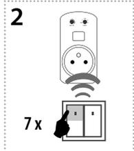
Seven presses of your selected button on the RF transmitter assigns the function ON/OFF (must be a lapse of 1s between individual presses).
