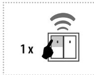
a) By pressing the programmed button for less than 0.5s, the light illuminates. By pressing the button shortly again, the light will continuously switch off for 3 seconds (at 100% brightness).
