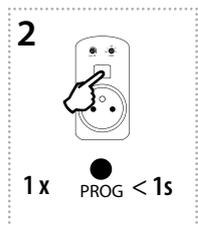
Pressing the programming button on the RFDSC-71 receiver for less than 1 second will finish the programming mode, this will reverse the memory function. The LED lights up according to the current pre-set memory function. The set memory function is saved. Every other change is made in the same way.
