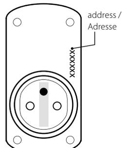
The address listed on the back of the socket is used for programming and controlling sockets by RF control units.
