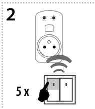
Assignment of the sunrise function is performed by five presses of the selected button on the RF transmitter (must be a lapse of 1s between individual presses).
