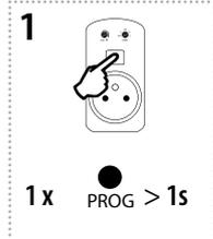
Press of programming button on socket RFDSC-71 for 1 second will activate socket RFDSC-71 into programming mode. LED is flashing in 1s interval.
