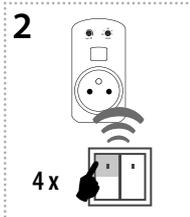
Four presses of your selected button on the RF transmitter assigns the function light scene 4 (must be a lapse of 1s between individual presses).
