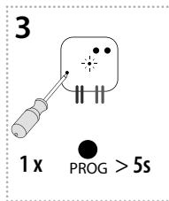
Press of programming button longer than 5 seconds, will activate actuator into timing mode. LED flashes 2x in each 1s interval. After releasing the button, the time of the sunset function begins to count down (period of complete dimming of the light).
