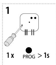
Press of programming button on receiver RFDEL-71B for 1 second will activate receiver RFDEL-71B into programming mode. LED is flashing in 1s interval.
