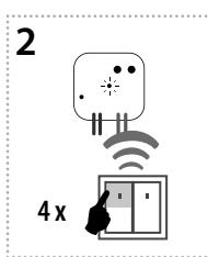
Four presses of your selected button on the RF transmitter assigns the function light scene 4 (must be a lapse of 1s between individual presses).
