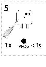
Press of programming button on actuator RFDEL-71B shorter than 1 second will finish programming mode. The LED lights up according to the pre-set memory function.
