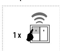
After pressing the programmed button, the light begins to illuminate in the programmed time interval in a range of 2 seconds to 30 minutes.
