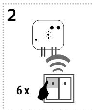
Assignment of the sunset function is performed by six presses of the selected button on the RF transmitter (must be a lapse of 1s between individual presses).
