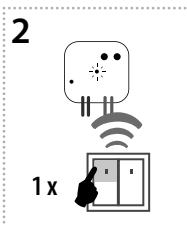
A press of your selected button on the RF transmitter assigns the function light scene 1.
