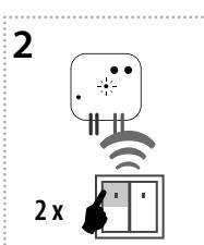
Two presses of your selected button on the RF transmitter assigns the function light scene 2 (must be a lapse of 1s between individual presses).
