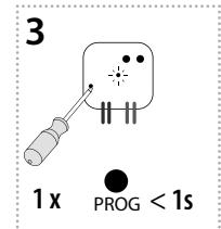
Press of programming button on actuator RFDEL-71B shorter than 1 second will finish programming mode. The LED lights up according to the pre-set memory function.
