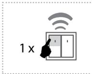
The dimmer output switches off by pressing the button.
