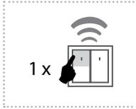
If the light is switched off, pressing the programmed button will switch it on. If the light is switched on, pressing the programmed button will switch it off.
