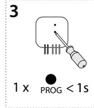
Press of programming button on actuator RFDAC-71B shorter than 1 second will finish programming mode. The LED lights up according to the pre-set memory function.
