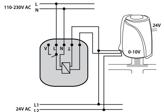
connection with a controlled dimmer (e.g. DIM-6) for dimming up to 2000VA
