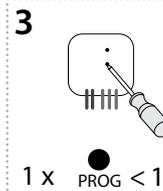
Press of programming button on actuator RFDAC-71B shorter then 1 second will finish programming mode. The LED lights up according to the preset memory function.
