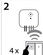
Four presses of your selected button on the RF transmitter assigns the function light scene 4 (must be a lapse of 1s between individual presses).
