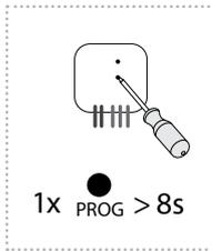
By pressing the programming button on the actuator for 8 seconds, deletion of one transmitter activates. LED flashes 4x in each 1s interval.
