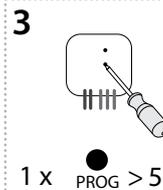
Press of programming button longer then 5 seconds, will activate actuator into timing mode. LED flashes 2x in each 1s interval. After releasing the button, the time of the sunrise function begins to count down (period of complete illumination of the light).
