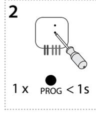
Pressing the programming button on the RFDAC-71B receiver for less than 1 second will finish the programming mode, this will reverse the memory function. The LED lights up according to the current pre-set memory function. The set memory function is saved.
