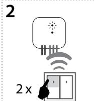
Two presses of your selected button on the RF transmitter assigns the function light scene 2 (must be a lapse of 1s between individual presses).
