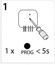
Press of Prog button for 3-5s will activate actuator RFDAC-71B into programming mode. LED is flashing in 1s interval.
