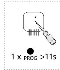
By pressing the programming button on the actuator for 11 seconds, deletion occurs of the actuator's entire memory. LED flashes 4x in each 1s interval.
