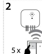
Assignment of the sunrise function is performed by five presses of the selected button on the RF transmitter (must be a lapse of 1s between individual presses).
