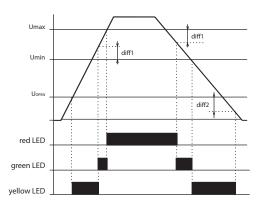
After connecting the supply voltage, the LED illuminates - the color corresponds to the voltage size of individual phases. If the phase voltage drops under 45 V (phase outage), the corresponding LED is not illuminated.
