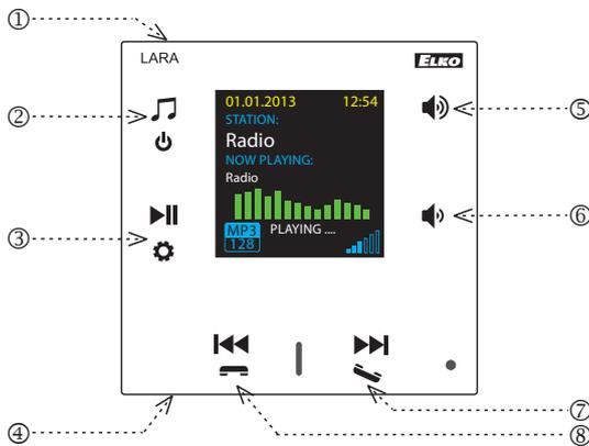
1. Hidden button RESTART - In the opening (in the upper part of the cover), for pressing use a thin object, i.e. a paper clip
