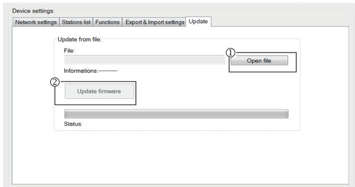
To update the FW in the LARA Radio device, it is first necessary to download the update file with the extension „\*.lfw“ from the address <http://www.elkoep.com/products/audiomedia/lara/radio/lara-radio-radio-mounted-in-the-wall-8295/>
