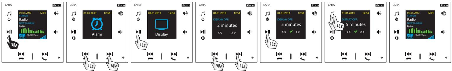
This concerns how long the display stays lit (10s, 20s, 30s, 1min, 2min, 5min). After this time expires the display goes out. It is activated by touching any button.
