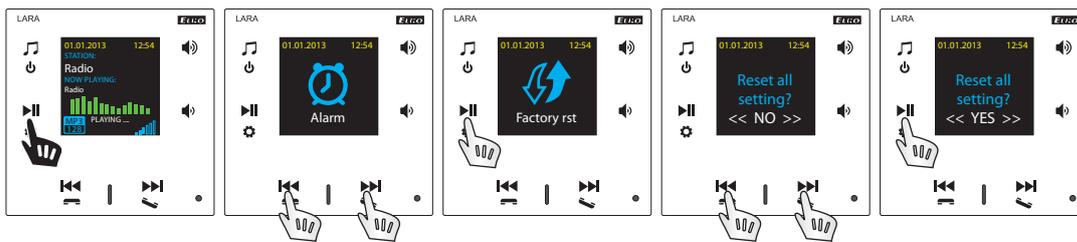
Through the settings menu, select „Factory rst“ - the IP address from the DHCP range will be set and the factory settings will be restored.
