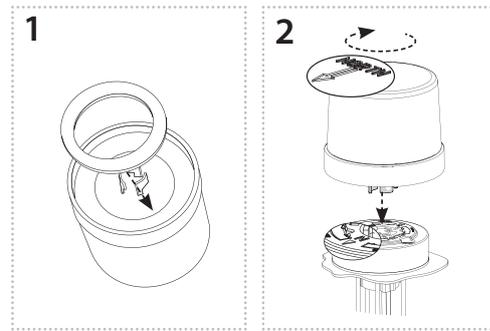
1. Remove the protective layer from the seal and glue it to the underside of the AirSLC-100 / NEMA.
