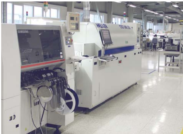
SMD production line
