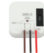
dimmer 3-wires (without NEUTRAL)
